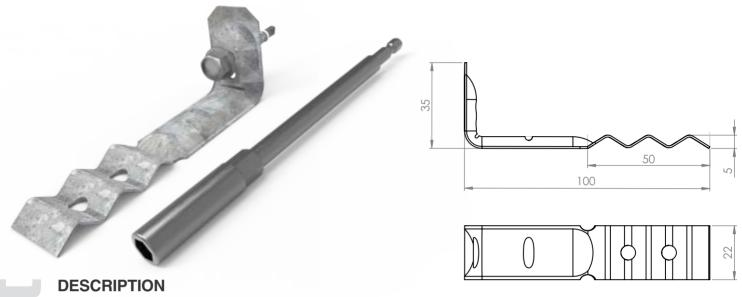
Stubi fast fix veneer tie for timber or steel stud construction Type A / 50mm cavity, Save installation time with the pre installed multi purpose screw for timer and metal framing. Supplied with the extra long driver bit to make installation easy as well as fast
